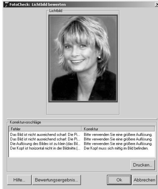
Figure 2: Software module for analysing the ICAO compliance rejecting a photograph due to deviation in facial pose
